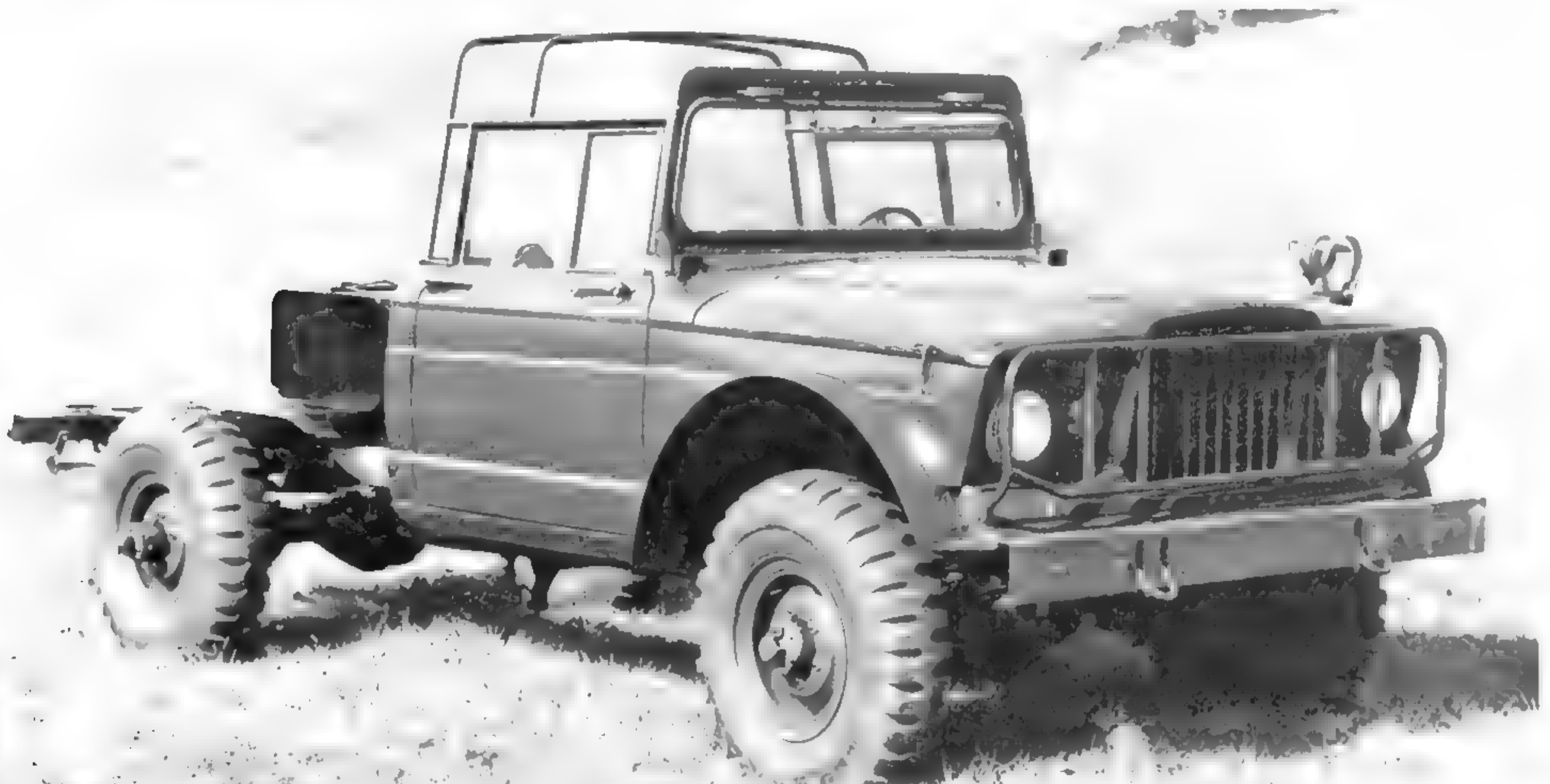
This is truly an M724 — simply a cab and chassis. The contact maintenance truck and the M726 were built on this chassis. (U.S. Army photo)
